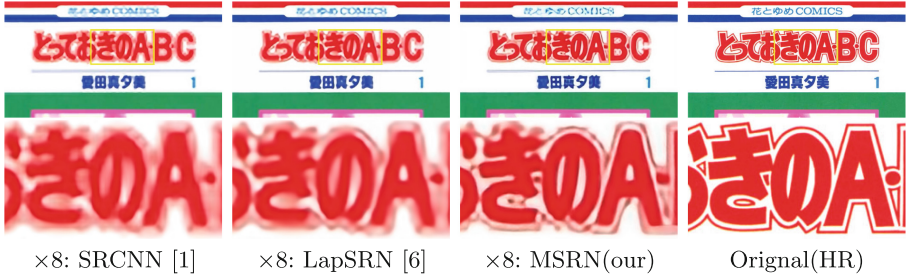
Fig. 7. Visual comparison of MSRN with other SR methods on large-scale ( \times 8 ) SR task. Obviously, MSRN can reconstruct realistic images with sharp edges.
