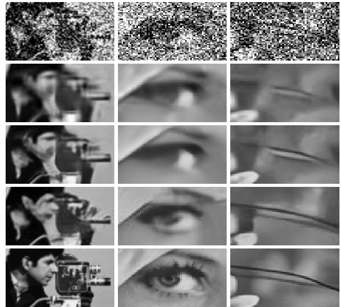
Fig. 11. Visual comparison on gray-scale images (noise level: \sigma = 75 ). Top to bottom: noisy image, denoised images by BM3D, denoised images by FFDNet, denoised images by MLEFGN (ours), and the ground truth.
